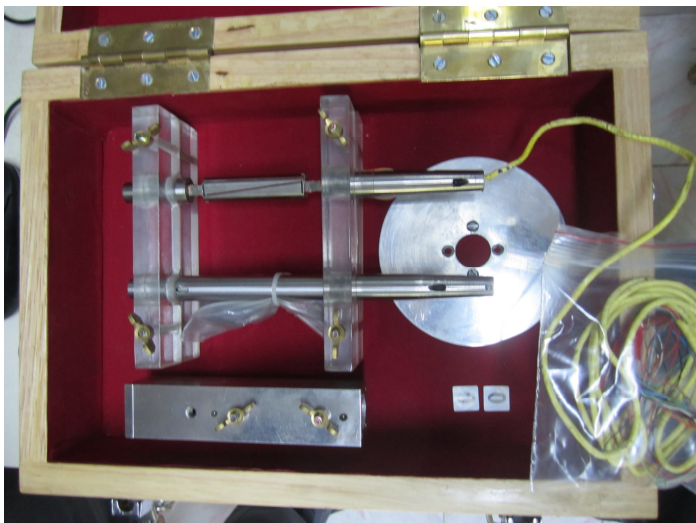
3 component and 6 component internal strain gauge balances for aerodynamic force and moment measurements
