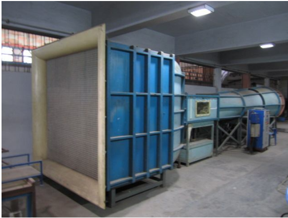
Subsonic wind tunnel facility with test section size 1' x 1' x 3'. Max. speed in test section 25 m/s.
