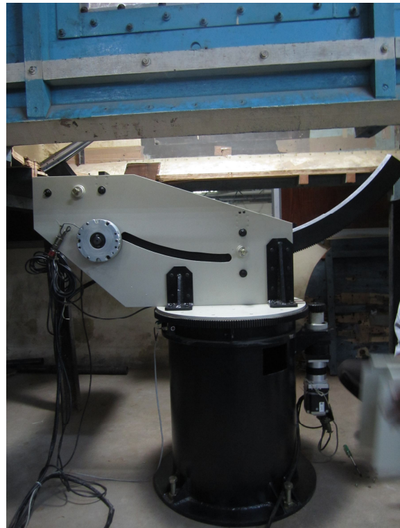
Electronically controlled angle of attack changing mechanism for aerodynamic models in wind tunnel test section
