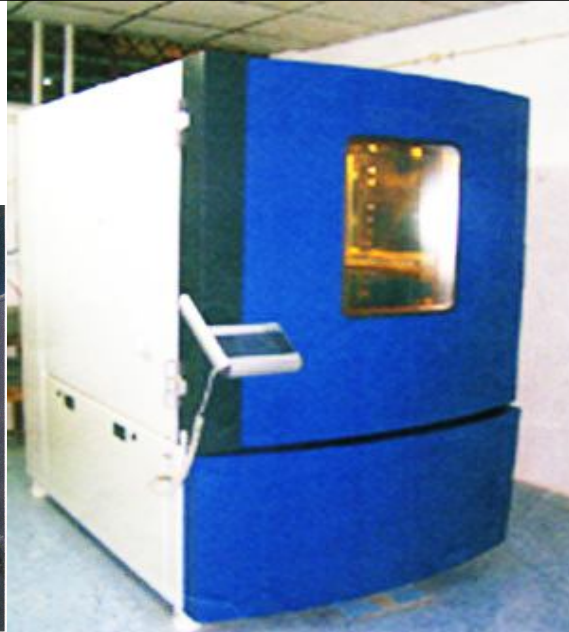
Weiss Technik make Climatic Chamber for studying environmental effects on materials for aero engines and airframes. Capacity 990 lr.
