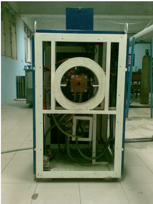
100 kW Plasma arcjet for thermal erosion Studies of aerospace materials (Max heat Flux is 10 MW/m 2 )
