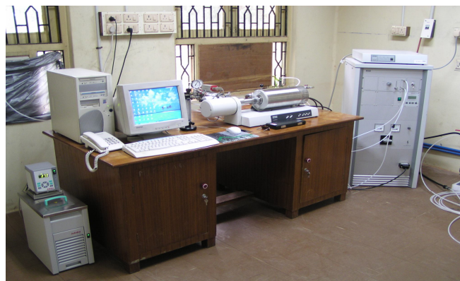
Dilatometer of NETZSCH make for thermal expansion studies of gas turbine blade and other aero engine & airframe materials up to 2000°C
