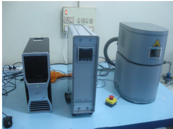
01dB Metravib make Dynamic Mechanical Analyzer 50N. Temperature range -120°C to 600°C. DM analysis is done for a variety of aerospace materials used for aero engines, airframes and seals.
