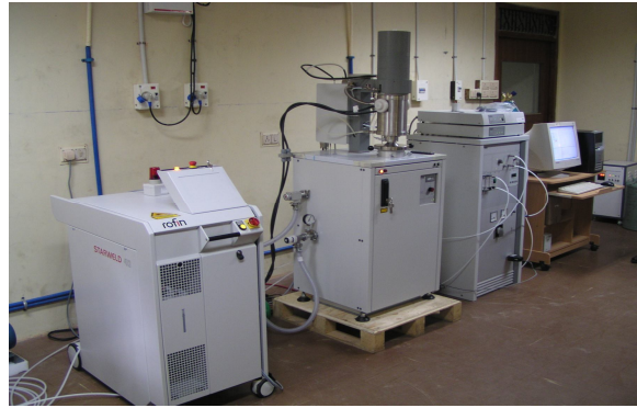
Netzsch make laser flash apparatus for measurement of thermal diffusivity of aerospace materials including gas turbine TBC. Measurements can be made up to 2000°C
