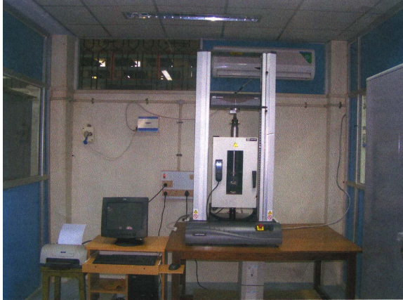
Instron make UTM type 3367 for testing materials for aero engines and airframes (-70 to 250°C) Capacity 3 ton.
