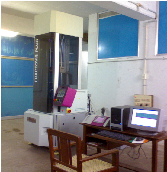
CEAST make Instrumented Impact Tester for determining impact strength of materials for aero engines and airframes.
