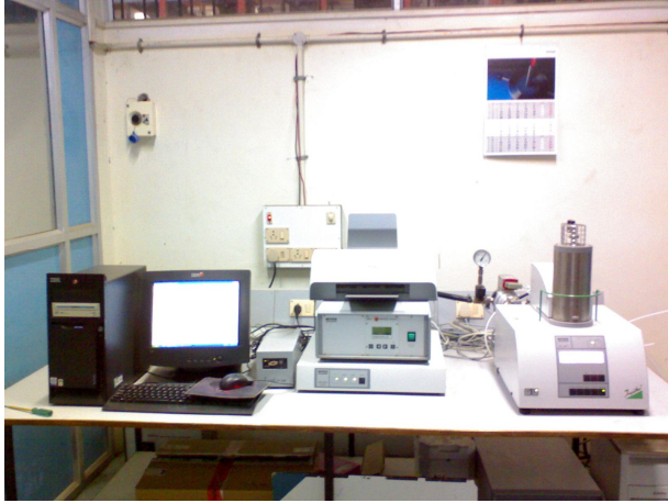
NETZSCH make simultaneous thermal analyzer for thermal analysis studies of aerospace materials up to 1400°C.
