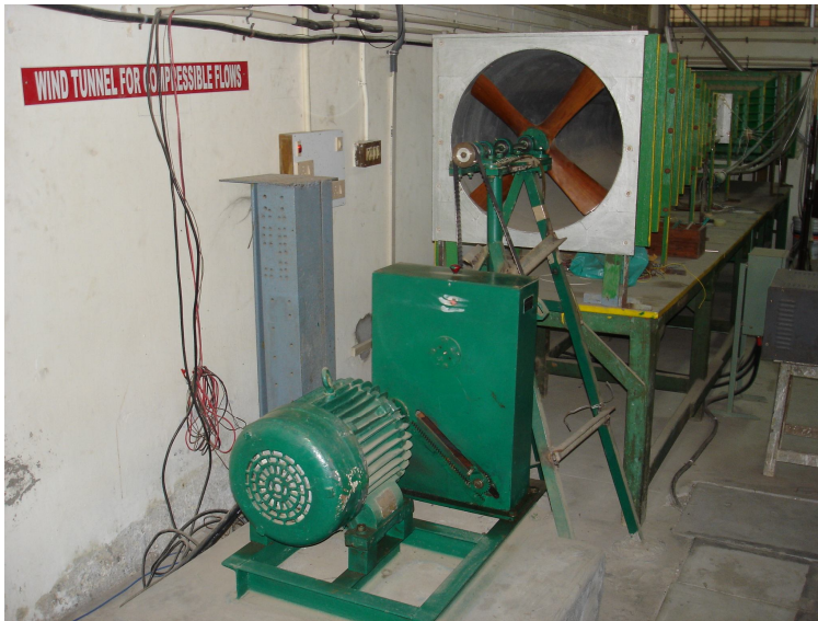
Propeller based table top air tunnel for internal flow studies such as diffuser and combustion chamber flows & recirculation zones behind flame holders with spray.
