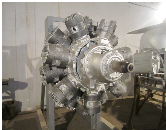
Double row radial piston engine for aircraft propulsion
