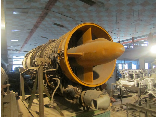
Axial flow compressor based gas turbine engine for aircraft propulsion
