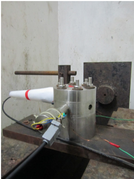
Ballistic evaluation unit for gas generating materials.
