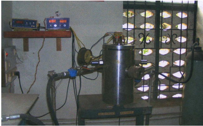
Strand burner facility for measurement of burning rates of filled viscoelastic materials for aerospace propulsion
