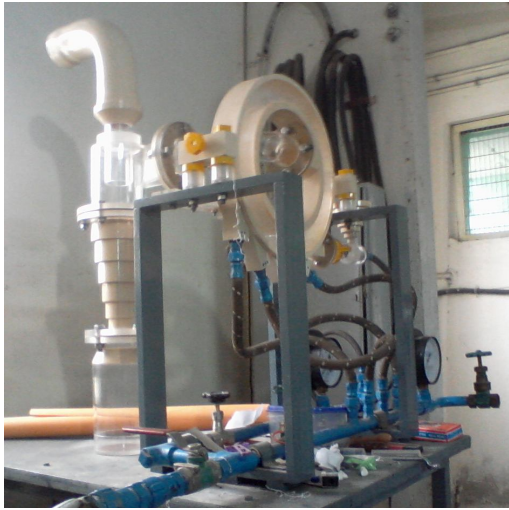
Pneumatic pulveriser for making fine powders for aerospace applications
