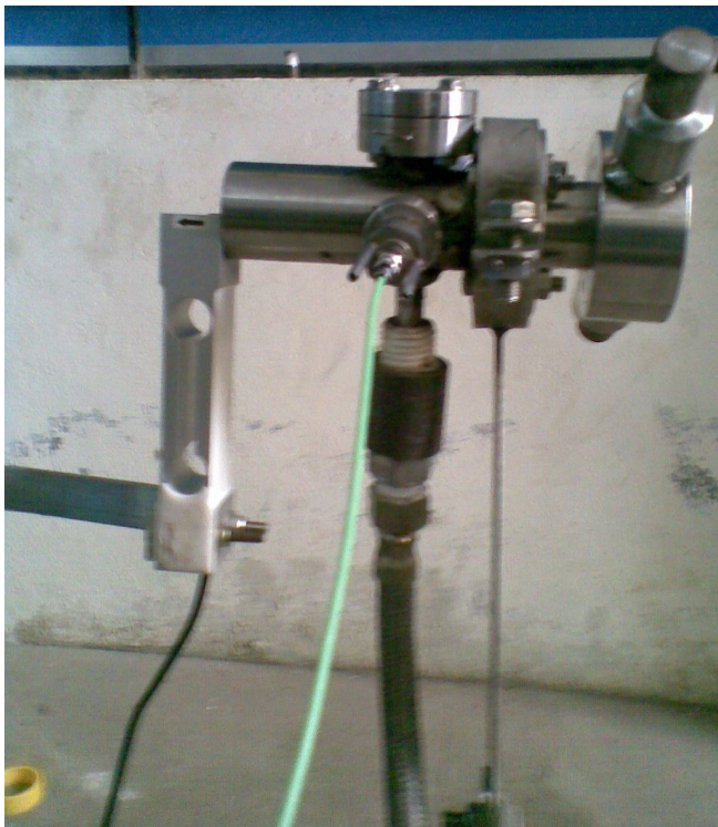
Mini solid thruster for performance studies of generator materials .
