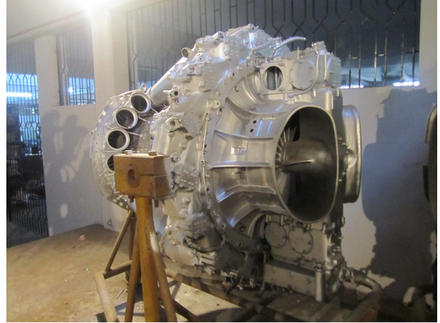
Centrifugal compressor based gas turbine engine for aircraft propulsion
