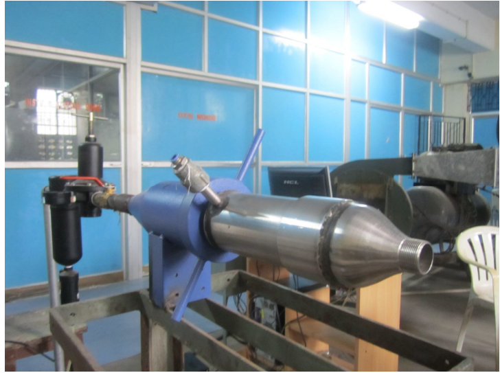
Experimental facility for high speed coaxial jet studies
