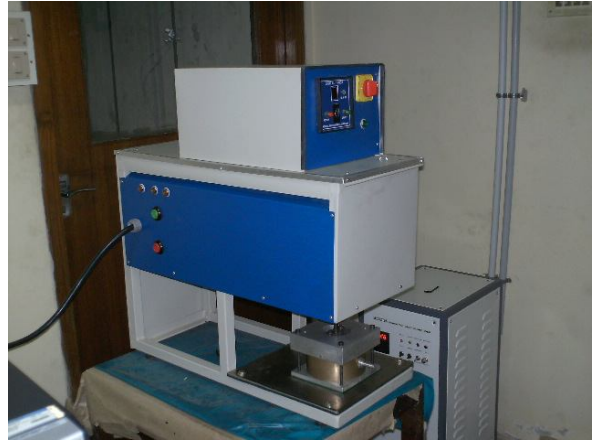
Mini mixer facility for preparing filled viscoelastic gels for aerospace applications.
