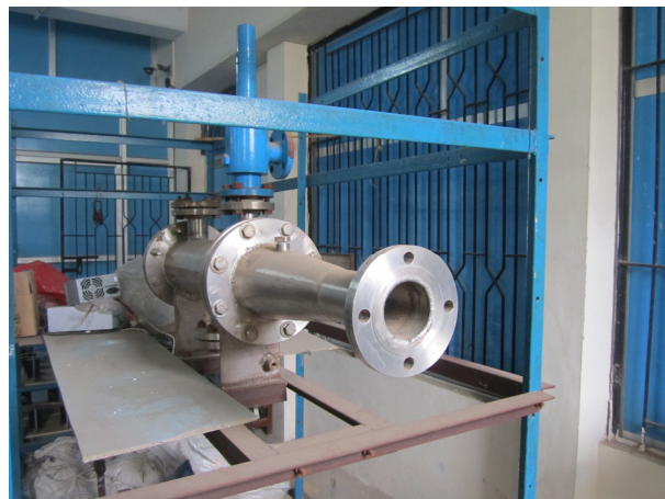
Oxalic acid based multi-tube heat exchanger for gas generator systems for aerospace applications.
